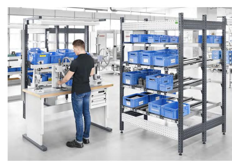
Make sure of optimum and efficient material provision in your manual assembly – with avero FIFO shelves! You remove the parts at the front of the assembly workstation, while the necessary supplies are continually provided from the back.
