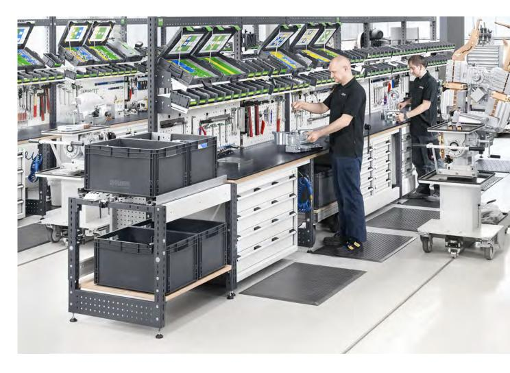
bott multi-workstations combine several workstations quickly and easily into assembly lines. The use of extension modules saves on components. The modular and sturdy set-up with freely combinable units also makes double-sided installation possible. If the same assembly line is built onto the back, up to 40% procurement costs can be saved.
